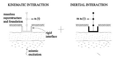
Figure 1. Decoupling of kinematic and inertial response (from Mylonakis, Nikolaou, & Gazetas, 2006)
