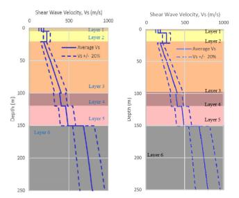
a) before densification of the sand b) after densification of the sand Figure 2. Average shear wave velocity measured at the new Baie-Saint-Paul hospital site
