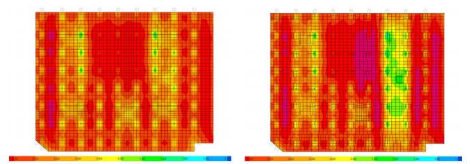
Figure 6. Comparison between new CNESST headquarters office building mat foundations stress state with (right) and without (left) soil liquefaction
