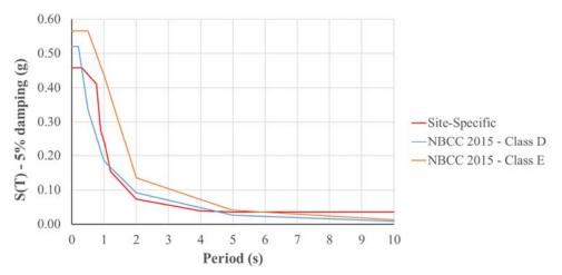
Figure 5. Site-specific response spectrum for the new CNESST headquarter project
